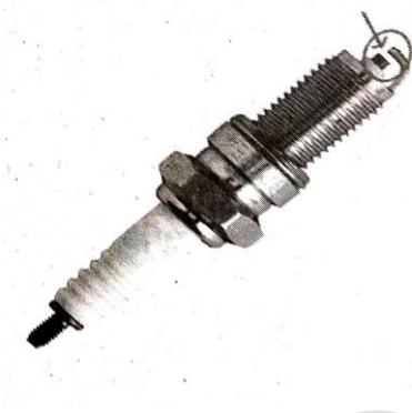
To create the spark, an electric field of magnitude  $3 \times 10^6 \text{ Vm}^{-1}$  is required. (a) What potential difference must be applied to produce the spark? (b) If the gap is increased, does the potential difference increase, decrease or remains the same? (c) find the potential difference if the gap is 1mm.
